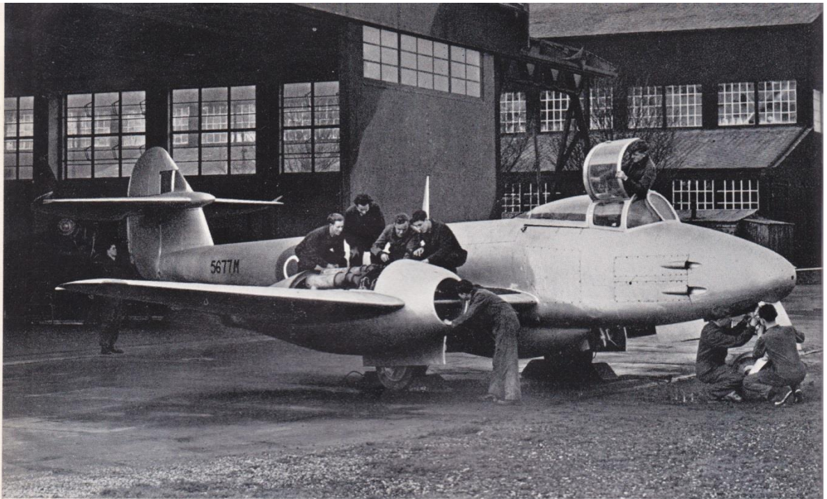
Aircraft engineering apprentices at Halton set to work overhauling a Meteor jet fighter.
