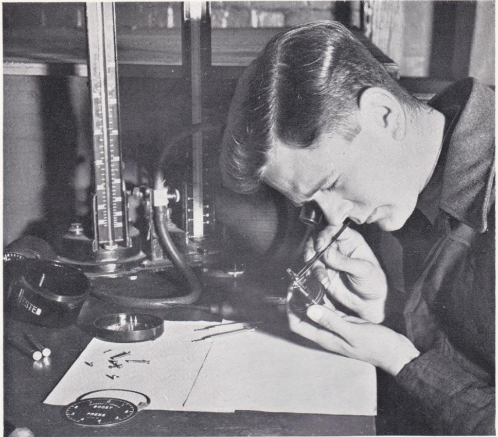
An instrument fitter concentrates as he adjusts a faulty boost pressure gauge.
